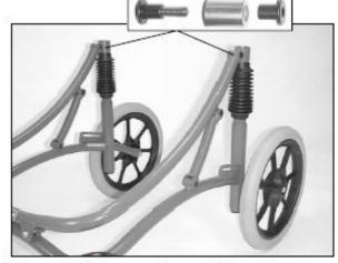
Mount tilt bar on down tubes: Place bushes in hinge eyes on down tubes, screw together with Allen screw heads and threaded rods.
