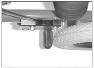
Mount brakes: Put bolts through slit on each side of under frame, put brake mechanism onto bolts, put screw nuts on.
