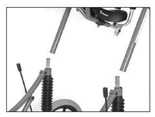
Mount top part on under frame: Place springs in top of down tubes. Slide top part into down tubes.
