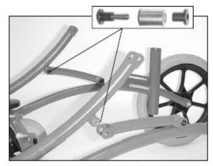
Mount tilt bar on under frame: Place bushes in hinge eyes on tilt bar, screw together with Allen screw heads and threaded rods.
