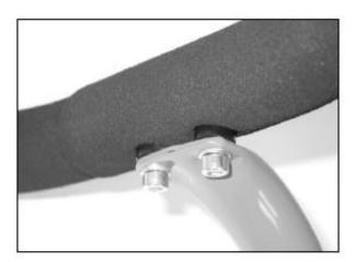
Mount trunk support: Trunk support and plastic washers are placed on top of top part, Allen screws with washers are screwed in from underside.
