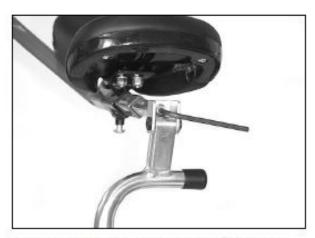
Mount rear stop: Slide rear stop tube into seat tube, tighten Allen screw.
