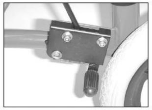
Adjust brakes so there is a gap of 3-5 mm between tyre and brake fitting.
