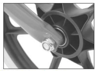
Mount rear wheels: Put bolt through wheel, slide bolt through under frame, screw nut on, put center cap on.
